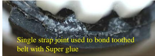
Single strap joint used to bond toothed belt with Super glue
