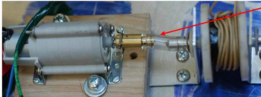
The coupling may be elastic, but to get it to bend, means large forces are placed on the delicate motor shaft!
