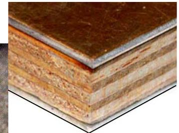
Aluminum epoxied to both sides of plywood which acts as a core
