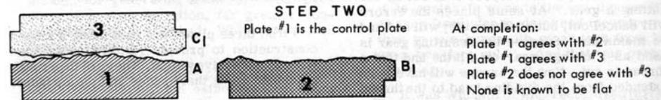
Fig. 15-5 At the completion of this step both #2 and #3 will have picked up #1's error.
