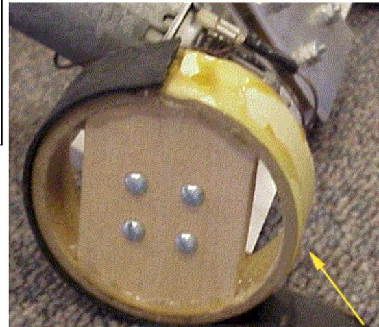
Improper surface preparation (rubber should be clean and rough), and the rubber should have been scarf joined
